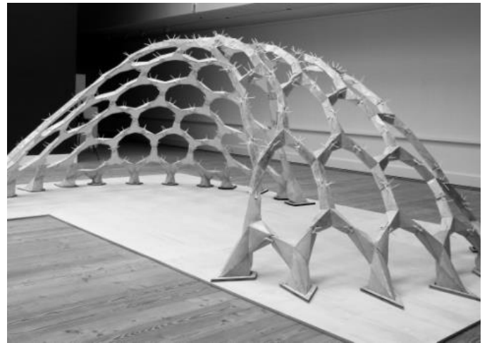
2 Concrete Grid-Shell Pavilion by Pigram, Larsen and Padersen (Pigram 2011)
