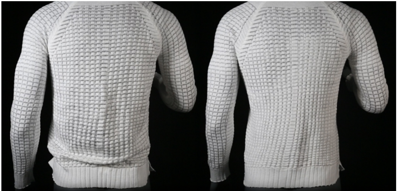
Figure 1: A textile garment shown before activation (Left) and after activation, demonstrating a tailored fit (Right).
