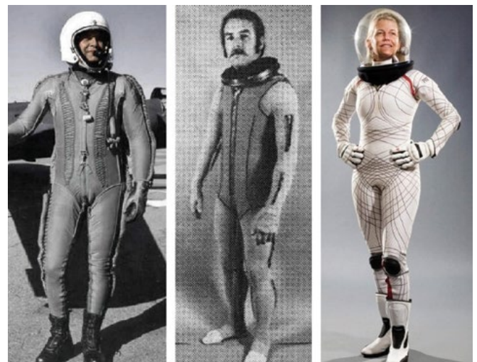
2 Evolution of Mechanical Counter Pressure (MCP) Suits including the David Clark MC-3 partial pressure suit for high-altitude flight (left), the 1960s Space Activity Suit (center), and the MIT BioSuit™ (right).
