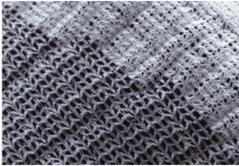
9 Knit zones enable longitudinal strain in the outer layer of non-elastic material (left) and innermost layer of elastic material (right).
