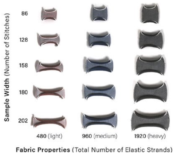
4 Knit cuff samples for collecting pressure data (left) and pressure measurements showing relationship between sample width, fabric properties, and reduction factor (right). As expected, pressure increases with a decreased sample width (i.e., an increased reduction factor), and pressure increases with heavier fabric properties, both due to increased fabric tension. These effects are consistent with the relationship defined by the hoop stress equation, which states that pressure is directly related to fabric tension and inversely related to cylinder radius (i.e., radius of the arm) (Schauss 2022).
